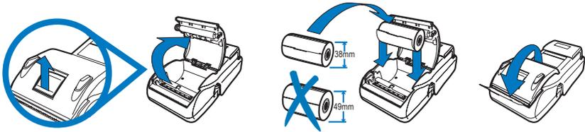
The paper that is used for VX680 has to be temperature sensitive (thermo) paper.
