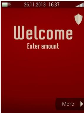
When the terminal starts up or is in the first position, "Welcome" displays on the screen. The terminal displays also the time, date, charging status and the GPRS signal.
